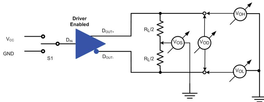
**Figure 1.** Driver  $V_{OH}$  and  $V_{OL}$  Test Setup
