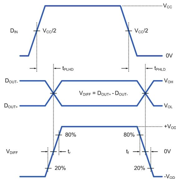
**Figure 3.** Driver Propagation Delay and Transition Time Waveforms
