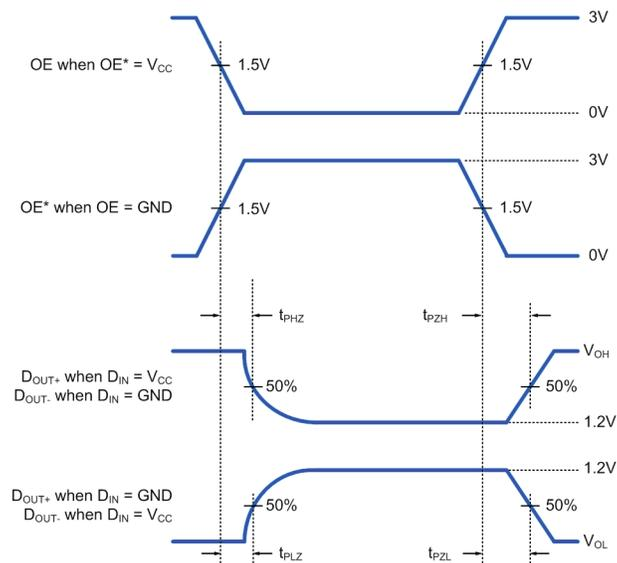
**Figure 5.** Driver High-Z Delay Waveforms
