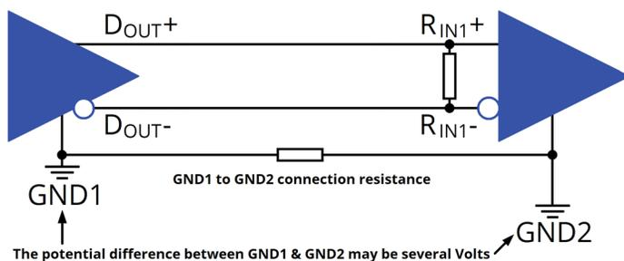
Figure 6. GND-potential difference
