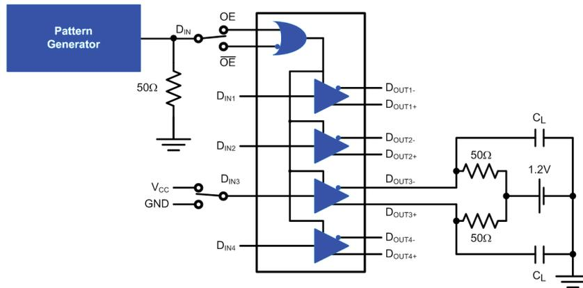
**Figure 4.** Driver High-Z Delay Test Setup
